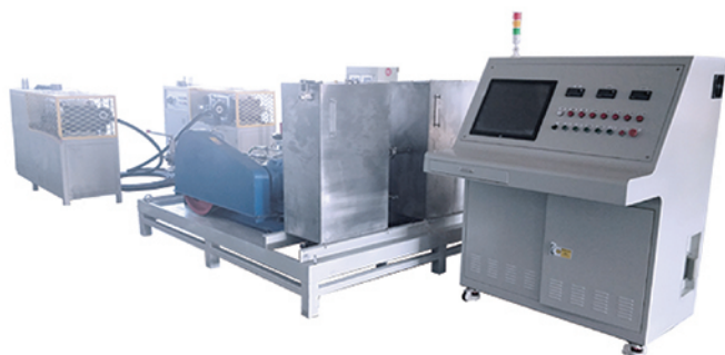
高压胶管脱芯试压试验台 Core-removing and Pressure-testing Test Bench for High-pressure Rubber Hoses
