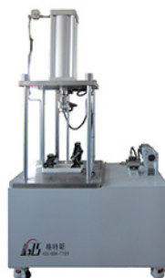
千斤顶动载/静载试验台 Dynamic Load/Static Load Test Bench for Jacks
